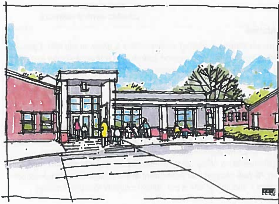
Architectural rendering of new entrance to Asa. Parent waiting area is to the right of the entrance. Behind the parent waiting area is an office with administrator eyes-on a double door entry system and additional support spaces.
